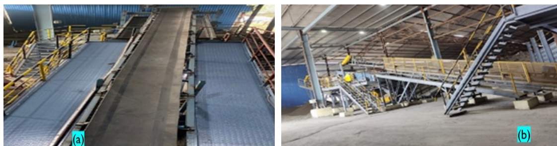
Figure 3. Left: Screen belt conveyor view, Right: Side view of double-decker vibrating screen capacity 200 t/day.
